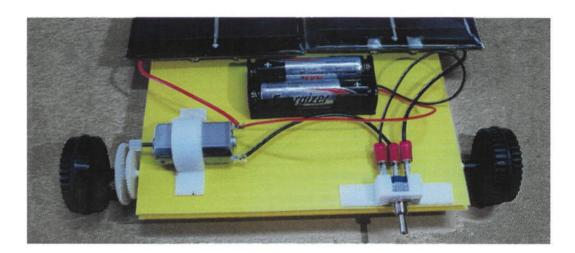
11. If you want to race the car down the track you will need to set up a method of keeping the car on the track. Some form of guide will be needed. This part is up to your imagination and is really important to help make your car go as fast as possible.
