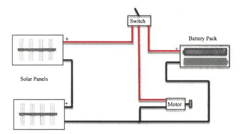
With the panels connected this way what is the output to the motor?
