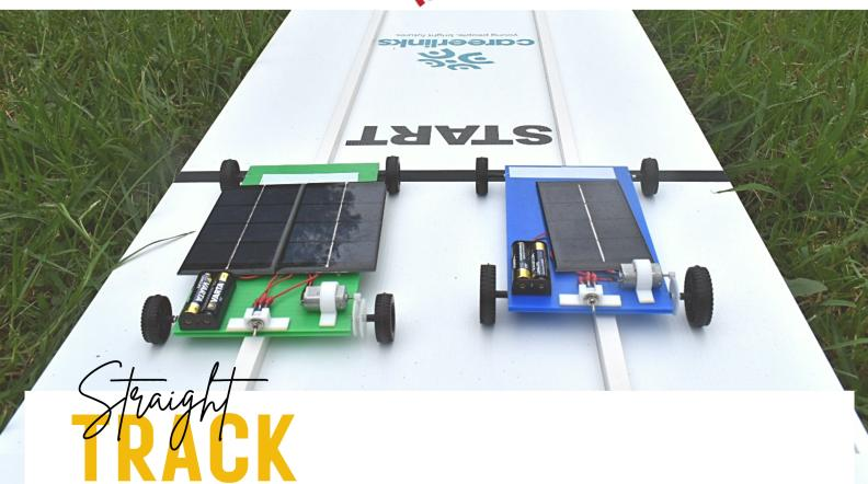
This race will be testing your car for **SPEED**. Your challenge apart from being first across the line is the accuracy of construction and strength. Alignment of wheels and motor are most important. The track is a straight line, so you need the car to track as straight as possible. Attention to detail and engineering are most important. Friction will be your biggest problem.
